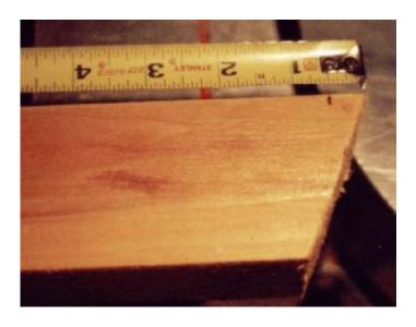
06) WITH YOUR SAW STILL SET AT 22 1/2 DEGREE; NIP THE CORNER OF THE LEG PIECES OFF OF ONE END. AS SHOWN IN THE PICTURE.
