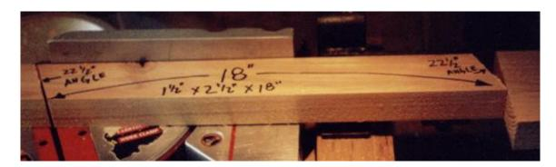
05) MEASURE 1/2" FROM ONE END OF EACH LEG, AND PLACE A MARK FOR CUTTING, AS SHOWN IN THE PICTURE.
